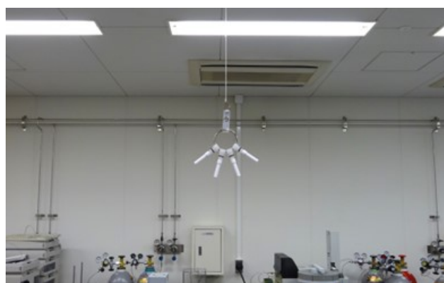
Fig. 2. Collection of gaseous chemical compounds in indoor air by using four kinds of PSD samplers.
