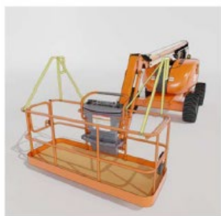
Figure 22 - Example of a physical barrier attached to the platform
