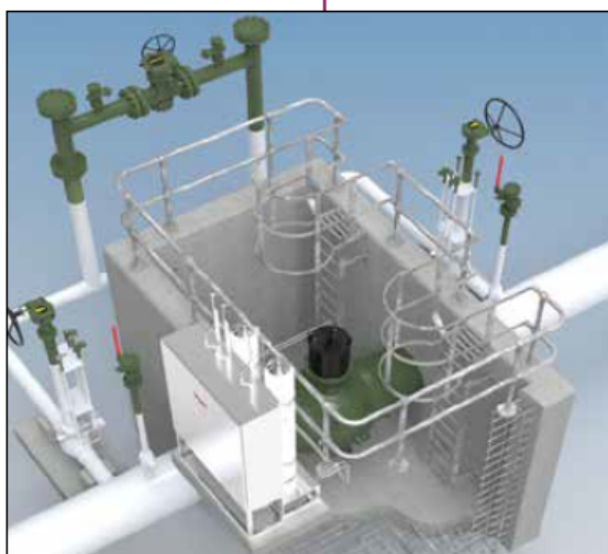
Figure 4 Railing without gated access
