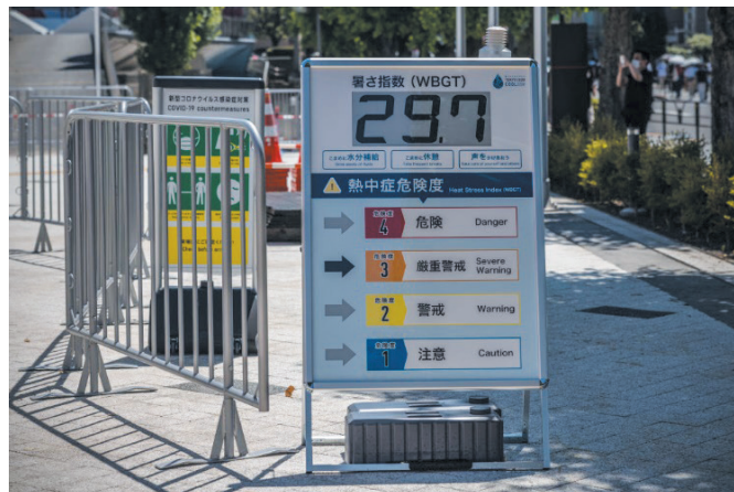
The signboard for Wet Bulb Globe Temperature (WBGT) and Heat Stress Index
