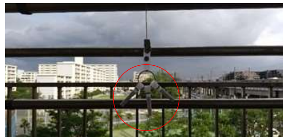
Fig. 3. Picture of the measurement of outdoor air using PSD samplers.
