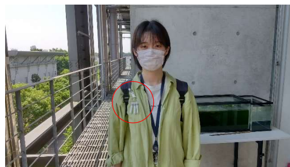
Fig. 4. Picture of the measurement of personal exposure using PSD personal samplers.
