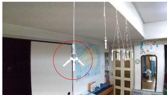
Fig. 2. Picture of the measurement of indoor air using PSD samplers.
