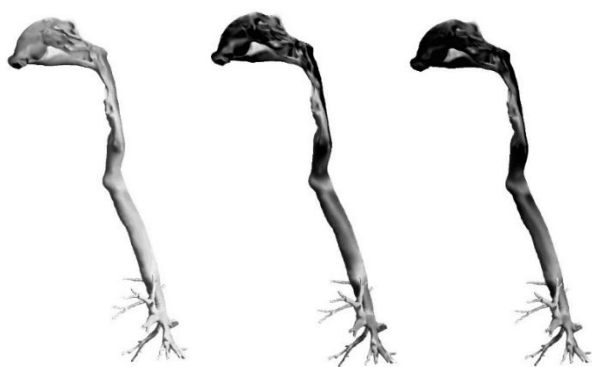
(1) t=40s (2) t=50sec (3) t=60sec Fig.6 Time series of ammonia concentration distribution in the respiratory tract model
