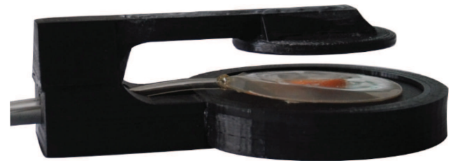
Figure 4: Prototype of the new blood pressure measurement device.
