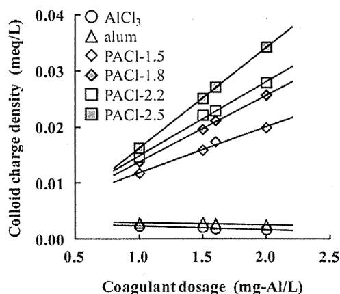
Figure 4 | Colloid charge densities of the coagulants as evaluated by the colloid titration technique.
