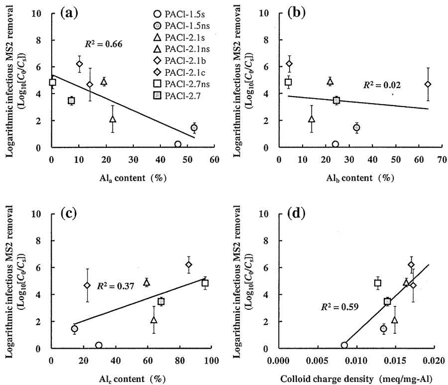
Fig. 8 – Relationship between infectious MS2 removal ratios and Al<sub>a</sub> (a), Al<sub>b</sub> (b), Al<sub>c</sub> (c), and colloid charge density (d). The source water was river water 2, and the coagulant dosage was 1.89 mg-Al/L. The pH of the treated water was approximately 8. Values are means (n = 3–4), and the error bars indicate standard deviations.
