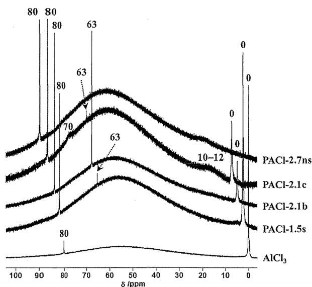
Fig. 7 —  $^{27}Al$  NMR spectra of coagulants used in the second set of experiments.
