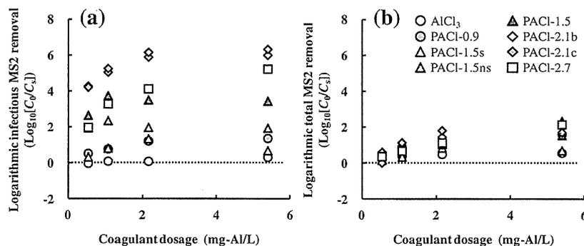
Fig. 9 – Effect of coagulant dosage on infectious MS2 removal as evaluated by the PFU method (a) and on total Q<sub>β</sub> removal as evaluated by the PCR method (b) after settling during the coagulation process. The source water was river water 3, and the pH of the treated water was approximately 8.
