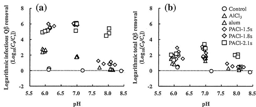
Fig. 1 – Effect of coagulant type on removal of infectious Q $\beta$  as evaluated by the PFU method (a) and on total Q $\beta$  removal as evaluated by the PCR method (b) after settling during the coagulation process. The source water was river water 1, and the coagulant dosage was 2.16 mg-Al/L.
