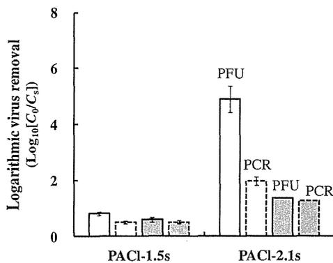
Fig. 2 – Comparison of Q $\beta$  (white) and MS2 (gray) removal ratios from treated water at around pH 8 after settling during the coagulation process. The source water was river water 1, and the coagulant dosage was 2.16 mg-Al/L. Values are means ( $n = 2-3$ ), and the error bars indicate standard deviations.
