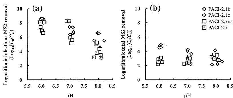
**Fig. 6** – Effect of the aluminum hydrolyte species in the coagulants on infectious MS2 removal as evaluated by the PFU method (a) and on total MS2 removal as evaluated by the PCR method (b) after settling during the coagulation process. The source water was river water 2, and the coagulant dosage was 1.89 mg-Al/L.
