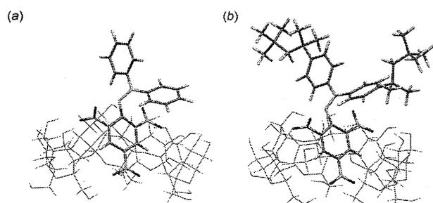
Fig. 2 Optimised structures of the inclusion complex of (a) DPPH<sup>•</sup> with β-CD and (b) DOPPH<sup>•</sup> with β-CD calculated by DFT (UB3LYP/3-21G:C-PCM solvation model parameterised for water).
