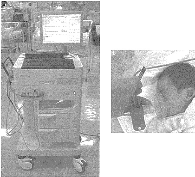
Fig. 1 (a) Aivision pulmonary function measuring system and (b) pneumotachometer with mask.
