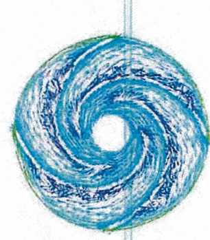
Fig. 17 Velocity vector near the back shroud of 1st impeller in Prototype 2 at Q=0.33Q_d and N=1150\text{rpm} , which correspond to Q=1\text{L/min} and N=4000\text{rpm} with the blood
