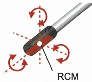
(c) Proposed device enables the 3 DOF desirable motion as (a) in the abdominal cavity
