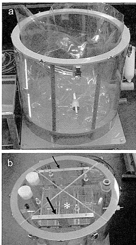
**Fig. 2.** Newly designed original inhalation chamber. a) Outer chamber and inner bag before top plate is in place. During operation, the space between the outer chamber and inner bag is negatively pressured to inflate the inner bag. b) Disposable top plate with tubing holes are placed on the chamber. The animal cages for 16 mice (asterisk) are suspended from the top place by a pair of hanger arms (arrows) (photo was taken without inner bag for better demonstration).
