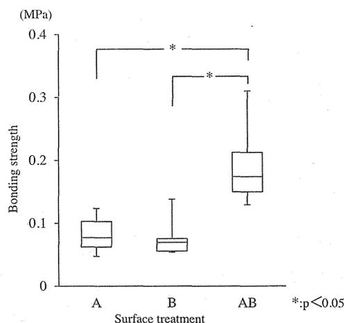
Fig. 1 – Tensile bond test (powder-water ratio: standard). (A) Air blow; (B) Surface baking; (AB) Alginate impression material bonding agent.
