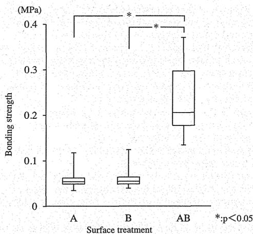
**Fig. 2 – Tensile bond test (powder–water ratio: 1.5×).** (A) Air blow. (B) Surface baking; (AB) Alginate impression material bonding agent.
