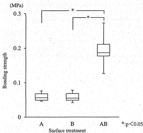
**Fig. 3 – Tensile bond test (powder–water ratio: 1.75×).** (A) Air blow; (B) Surface baking; (AB) Alginate impression material bonding agent.
