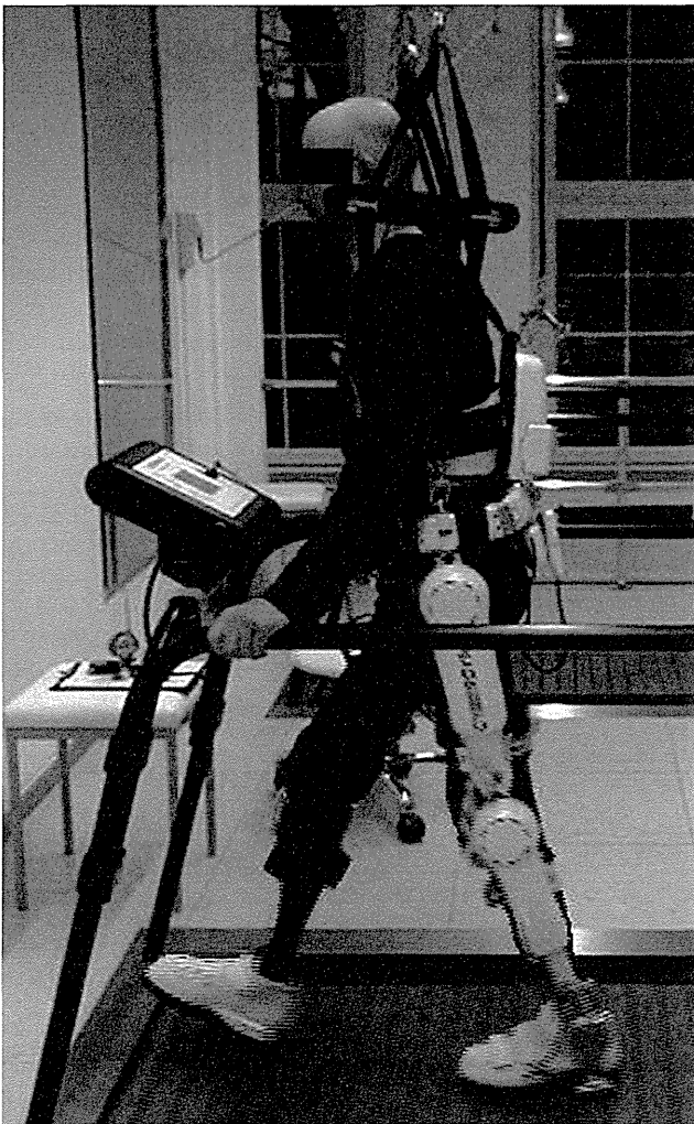
Fig. 2. Patient performing treadmill locomotion training with body weight support and hybrid assistive limb exoskeleton.
