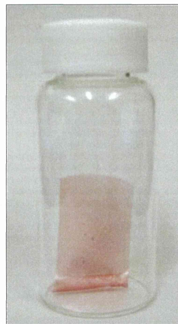
Figure 1. Photoelectric dye-coupled polyethylene film (OURePT TM ): a novel type of retinal prosthesis.
