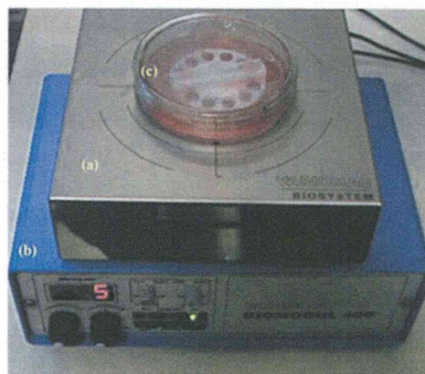
図 B-7. Photograph of the device for sliding culture. (a) Magnetic stirrer, (b) control unit and (c) poly(MPC) coated dish
