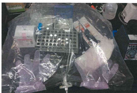
Figure 18 Endotoxin measurement system by using clean bag.
