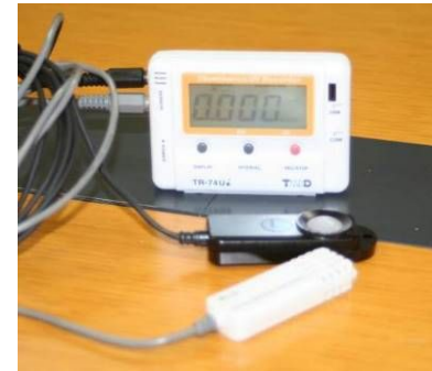
Illuminance UV Recorder (温度、湿度、照度)
