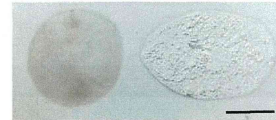
Fig. 6 – Detached white-colored silver metal heated at 700 °C on zirconia plate. Left: solid metal; right: porous metal made from silver clay with 30% hydrogen peroxide. Solid metal could be detached from zirconia plate easily (A), however, strong force was needed to detach the porous one from zirconia plate with remaining of porous one (B). Black bar indicates 1 cm
