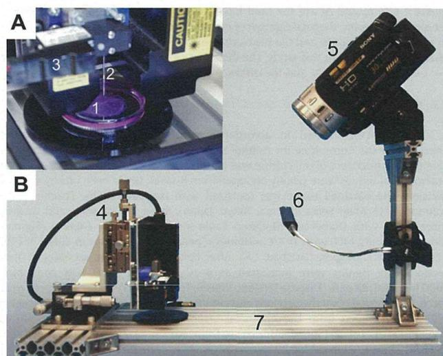
**Fig. 2.** Experimental setup for assessing the wettability of cultured cells. (A) Close-up view of air-jet application unit. (1) Cultured cells on a cell-culture substrate, (2) 0.5-mm-inner-diameter Air-nozzle, and (3) A electrical solenoid valve. (B) General view of experimental setup. (4) A position adjuster for x-y-z-axes directions, (5) A full-hivision movie camera, (6) An LED illumination, and (7) A home-made base-plate made of aluminum frames.
