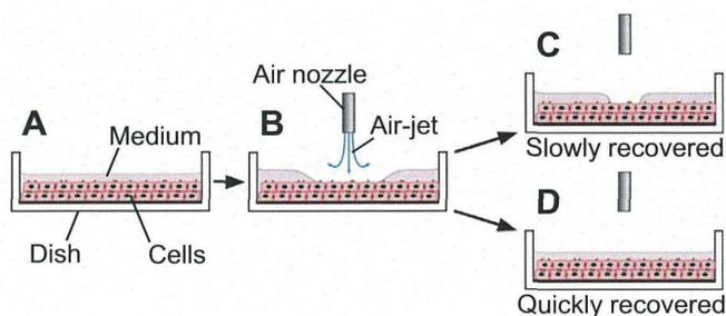
**Fig. 1.** Procedure of wettability assessment of cultured-cell surface. (A) Confluent cells on a cell culture dish were covered with a constant volume of culture medium. (B) Air-jet was given from an air-nozzle to the surface of culture medium, and the culture medium was squeezed by the air-jet. (C) In the case of hydrophobic surface, the squeezed area of culture medium was still remained. (D) On the other hand, in the case of hydrophilic surface, the culture medium recovers quickly.
