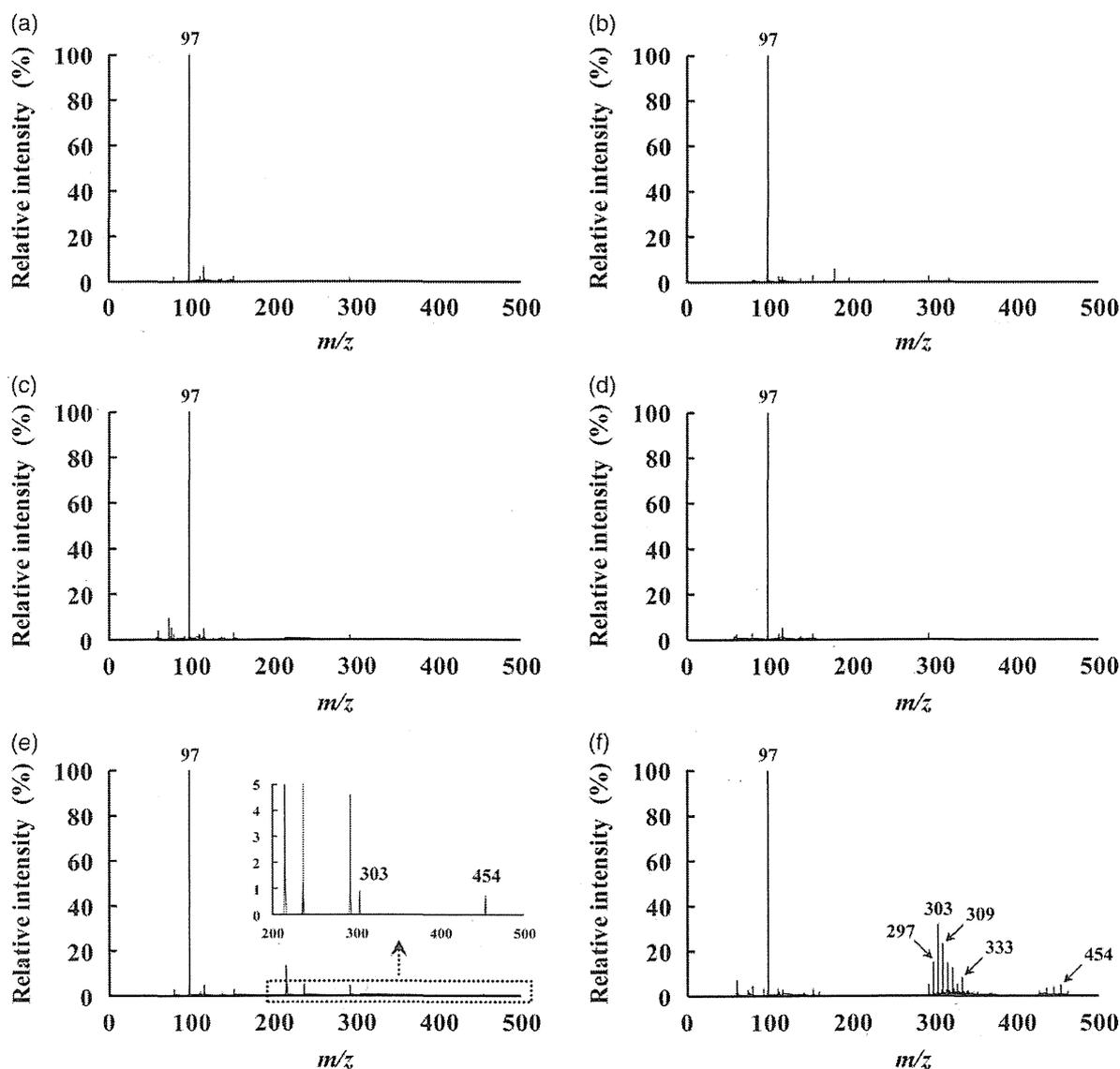
Figure 3 | ESI-TOF-MS spectra of coagulants: AlCl<sub>3</sub> (a), alum (b), PACl-1.5 (c), PACl-1.8 (d), PACl-2.2 (e), and PACl-2.5 (f).
