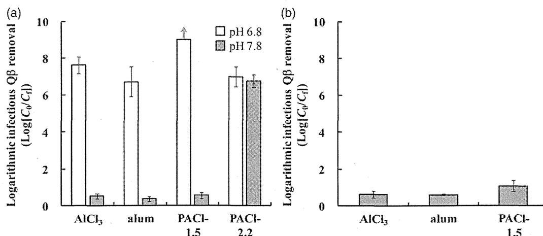
**Figure 1** | Effect of coagulant type on removal of infectious Q $\beta$  by the in-line coagulation—ceramic MF process as evaluated by the PFU method. Source water was river water 1. Coagulant dosage was 1.08 (a) or 2.16 (b) mg-Al/L. Values are filtration time-averaged removals, and the error bars indicate standard deviations. The absence of a bar indicates that the Q $\beta$  concentrations were below the quantification limit in the treated water.
