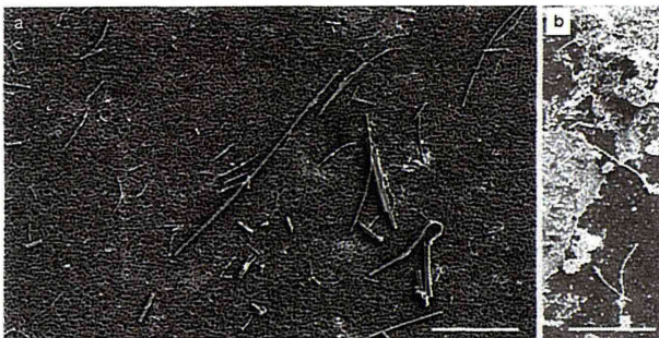
Fig. 10. T-CNT recovered from the mouse lung. a) SEM of the sediment of the dissolved lung of a mouse exposed to T-CNT in an inhalation chamber 2 hr a day for 5 days, \times 2,000 . Long and short single fibers are shown to be inhaled (treated with solution containing EDTA and ascorbic acid). b) SEM of a same sample treated without EDTA and ascorbic. The debris covering the fibers is considered to be iron-based amorphous substances soluble to EDTA, \times 2,000 . Ascorbic acid was found to be effective in keeping iron ions to be bivalent (ferrous) and soluble. (scale bars are 10 \mu\text{m} )
