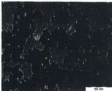
Fig. 1. Representative transmission electron microscopic view of magnetite nanoparticles. The estimated primary particle size is about 5–15 nm in diameter.
