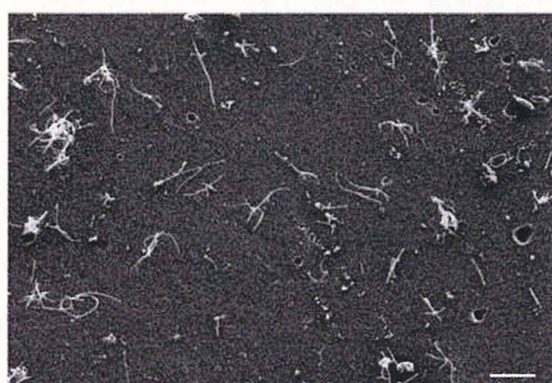
Fig. 7. T-CNT aerosol at a concentration of 1 mg/m 3 in the main chamber was collected on the Anodisc filter (5 L/min for 3 min). SEM × 1,000. (scale bar is 10 μm)
