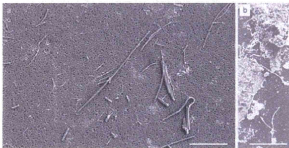
Fig. 10. T-CNT recovered from the mouse lung. a) SEM of the sediment of the dissolved lung of a mouse exposed to T-CNT in an inhalation chamber 2 hr a day for 5 days, \times 2,000 . Long and short single fibers are shown to be inhaled (treated with solution containing EDTA and ascorbic acid). b) SEM of a same sample treated without EDTA and ascorbic. The debris covering the fibers is considered to be iron-based amorphous substances soluble to EDTA, \times 2,000 . Ascorbic acid was found to be effective in keeping iron ions to be bivalent (ferrous) and soluble. (scale bars are 10 \text{ } \mu\text{m} )
