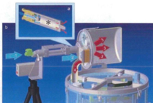
Fig. 3. A scheme of direct injection aerosol generation system. a) Upper inset shows the cut section of the injection cartridge (capacity; 23.5 ml). A slide valve opens when the cartridge is loaded to the subchamber. A measured amount of dispersed MWCNT is preloaded inside the cartridge shown in asterisk. b) Compressed air (Blue arrow 1) blows out the MWCNT through four small outlets of the cartridge into the subchamber (red arrows 3), where main flow air from the HEPA filtered inlet (blue arrow 2) mixes in. The air with the aerosol goes down the connection pipe to the main chamber (red arrow 4).
