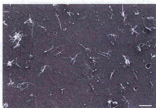
Fig. 7. T-CNT aerosol at a concentration of 1 mg/m 3 in the main chamber was collected on the Anodisc filter (5 L/min for 3 min). SEM x 1,000. (scale bar is 10 μm)
