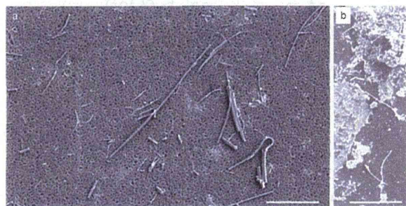
Fig. 10. T-CNT recovered from the mouse lung. a) SEM of the sediment of the dissolved lung of a mouse exposed to T-CNT in an inhalation chamber 2 hr a day for 5 days, \times 2,000 . Long and short single fibers are shown to be inhaled (treated with solution containing EDTA and ascorbic acid). b) SEM of a same sample treated without EDTA and ascorbic. The debris covering the fibers is considered to be iron-based amorphous substances soluble to EDTA, \times 2,000 . Ascorbic acid was found to be effective in keeping iron ions to be bivalent (ferrous) and soluble. (scale bars are 10 \text{ } \mu\text{m} )
