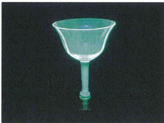
Fig. 4. (Color online) Uranium glass which illuminating fluorescence under UV light exposure.
