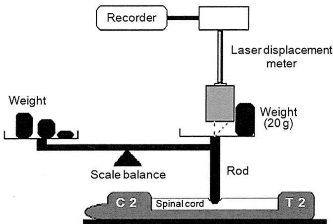
**Fig. 1.** Schematic drawing of the indentation test of the spinal cord. A rod of 5 mm in diameter was placed on the spinal cord. The rod was connected with a pan of a scale balance. Varying the weight on the other scalepan, the indentation of the rod on the spinal cord was measured with a laser displacement meter as a vertical displacement of the pan.
