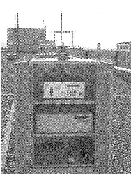
FIG E2. Automatic apparatus for measuring JCP levels. The pictured equipment automatically counts the amount of airborne JCP and transfers the data to a central office through telephone lines. This machine is based on a new laser particle counter methodology to measure the optical properties and hydrodynamic characteristics of pollen.
