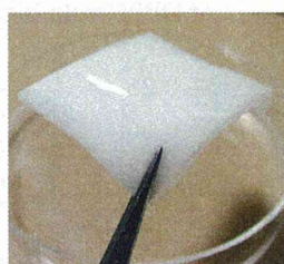
Fig. 2 PVA hydrogel prepared by freezing-thawing method
