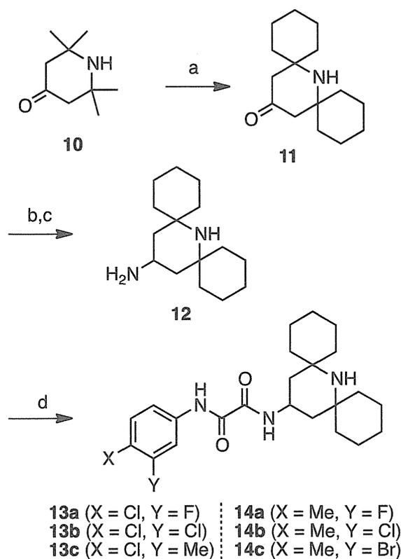
**Scheme 2.** Reagents and conditions: (a) cyclohexanone, NH<sub>4</sub>Cl, DMSO, 60 °C; (b) *p*-methoxybenzylamine, NaBH<sub>3</sub>CN, MeOH, then 1 M TMSBr in TFA; (c) CAN, CH<sub>3</sub>CN/H<sub>2</sub>O (v:v = 2:1); (d) **6** or **7**, Et<sub>3</sub>N, EtOH, 150 °C, microwave.
