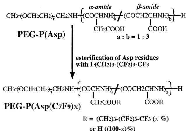
Fig. 2. Synthesis of the fluorocarbon-containing block copolymer PEG-P(Asp(C7F9))<sub>x</sub>.
