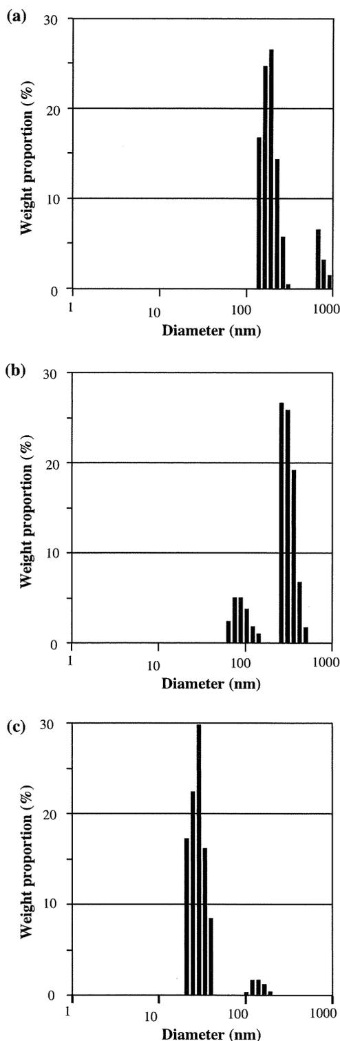
**Fig. 3.** Diameter distribution of PFC5-containing nano-emulsions (a and b) forming from PEG-P(Asp(C7F9)59) and empty polymeric micelle (c) measured by means of DLS. (a and b) are of different batches but prepared in the same conditions.
