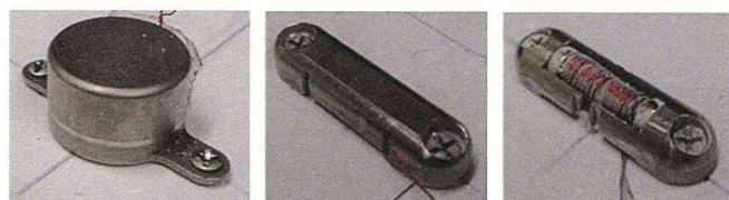
(a) Bonebridge (b) Hinge type (c) Spring type Fig. 2 Transducers.
