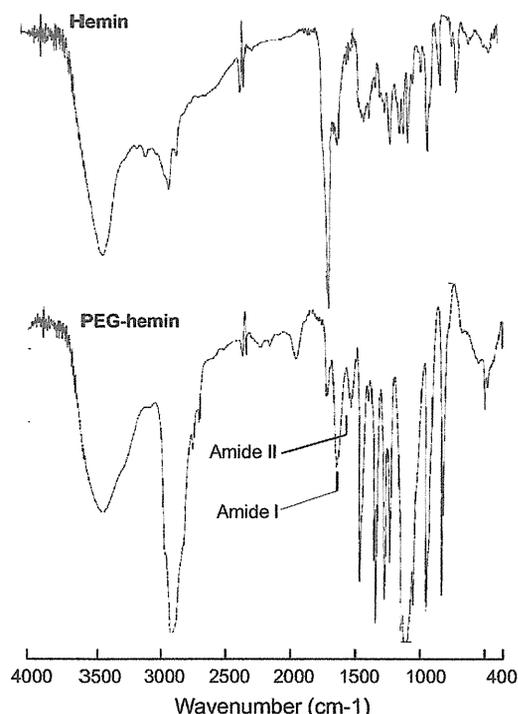
Fig. 1. IR spectra of hemin and PEG-hemin. Amide I ( $1654\text{ cm}^{-1}$ ) and amide II ( $1542\text{ cm}^{-1}$ ) were clearly observed in PEG-hemin, which suggested an amide bond formation between hemin and PEG through bis-(ethylenediamino) hemin.
