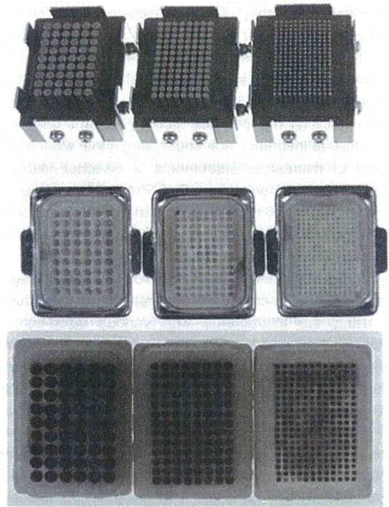
Figure 2 Tissue microarray gauges, prefabricated recipient blocks with holes, commercially available, and embedded blocks from top to bottom. The core diameters are 3 mm, 2 mm, and 1 mm in diameter (left to right).
