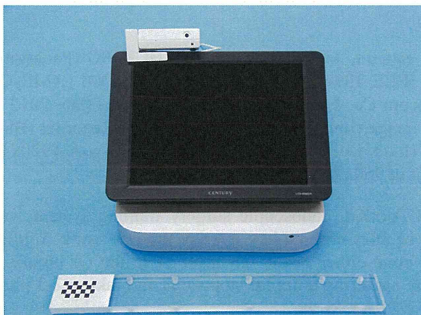
3) Ultrasound – endoscopic image overlay system. A USB camera and a movie file were used instead of endoscope and echo images.
