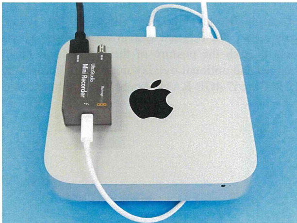
1) Image processor for stereo endoscope. Small gray box is UltraStudio Mini Recorder.
