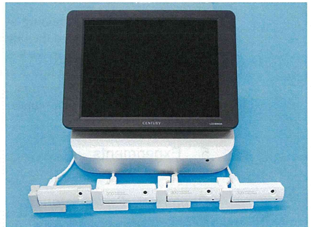
2) Four USB-camera event detection and recorder
