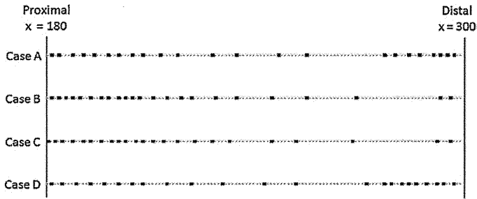
Fig. 8. Strut distribution along the aneurysm neck for the four initial stents, after the optimization process.
