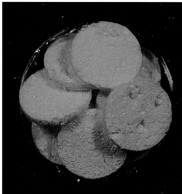
FIG. 1. A picture of OCP/collagen disks. OCP/collagen disk is 9 mm in diameter and 1 mm thick. OCP, octacalcium phosphate.
