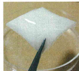
Fig. 2 PVA hydrogel prepared by freezing-thawing method
