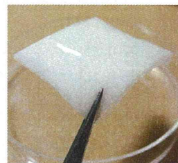
Fig. 2 PVA hydrogel prepared by freezing-thawing method
