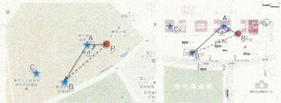
Fig. 2. Positioning in an inconsistent map (right) using positions of POIs (left figure shows the positions in the real world).
