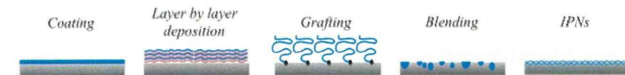
Figure 2. Schematic of molecular designs (a) and surface modification (b) performed with MPC polymer science.
