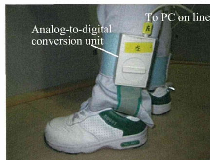
(c) Fitted measuring equipment on an examinee's leg
