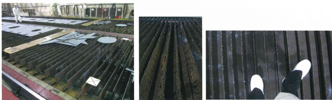
(a) Slat type surface plate for NC plasma cutting machine
