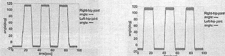
(a) The trajectories when LoMS was outside the MRI environment: The rotation angle of the joint is limited from -15 to 110[deg].
