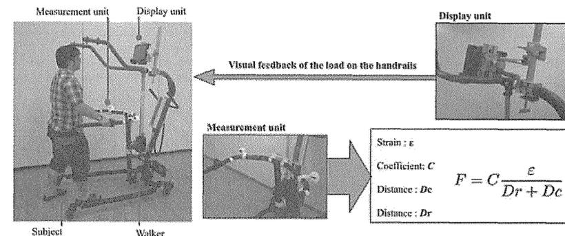
Fig. 2: The developed system for giving the feedback of the loads on handrails to the trainee during gait training. The trainee can know the loads information by looking at the display unit.
