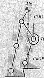
Fig. 7. The force vector from the COG and the force vector from CoGRF during moving upward. These vectors are considered to be in the same distance from the knee joint in the sagittal plane.
