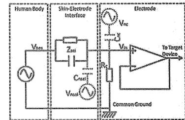
Fig. 1. Electrode equivalent circuit
