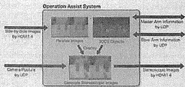
Fig. 6. The information flow of Operation Assist System. The system receives the information of the camera posture and parallax image from motion 3D camera system. Stereoscopic images are generated using camera posture and 3DCG objects. Then, those images are sent to 3D monitor using HDMI. In addition, position of end effector is sent to master system and slave system using UDP protocol.
