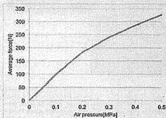
Fig. 13. Relationship between average force generated by FRF generator and air pressure: The generated force is proportional to the supply pressure.
