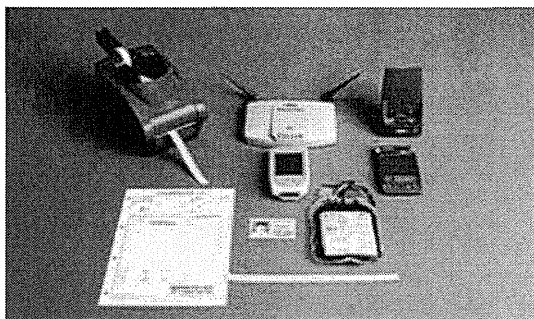
Fig. 2 Total equipment for the barcode patient-blood unit identification system, including wristband with barcode, label printer, and hand-held computer with barcode reader.
