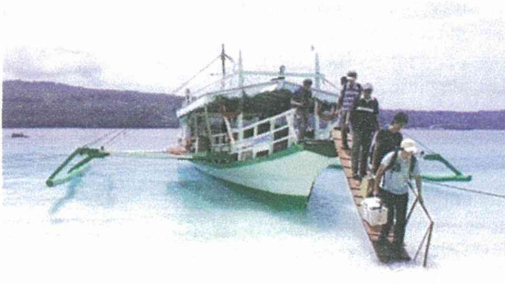
This picture shows the bat team disembarking from the boat. Take note that boats with outrigger have a shallow draft enabling them to come closer to shore without need for piers.
